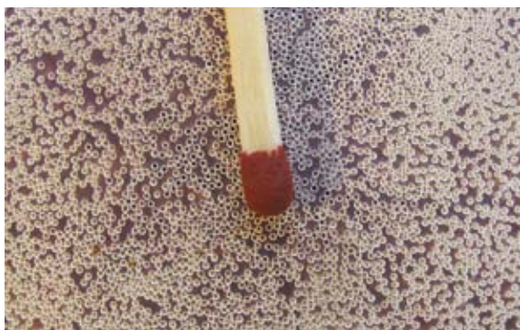
PPO Fibres 0.5mm diameter
